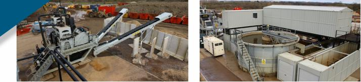
The Compact CSP12 is a modular sand recovery unit which is designed to be both cost and energy efficient. The cyclones remove clays, silts and slime from sand and bring it into specification. It offers exceptional performance, producing two grades of sand.
