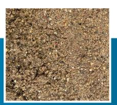
0 - 2mm Fill sand It is most commonly used for plastering and rendering sand, pipe bedding and mixed with cerement to create floor Screed.
