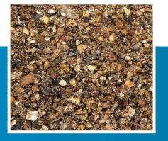
0 - 4mm Grit sand This is used for making concrete; also used as a general drainage fill for construction projects.
