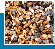
10 - 20mm Aggregate This is most commonly used for surfacing driveways and paths, but also serves as a drainage material for construction projects.
